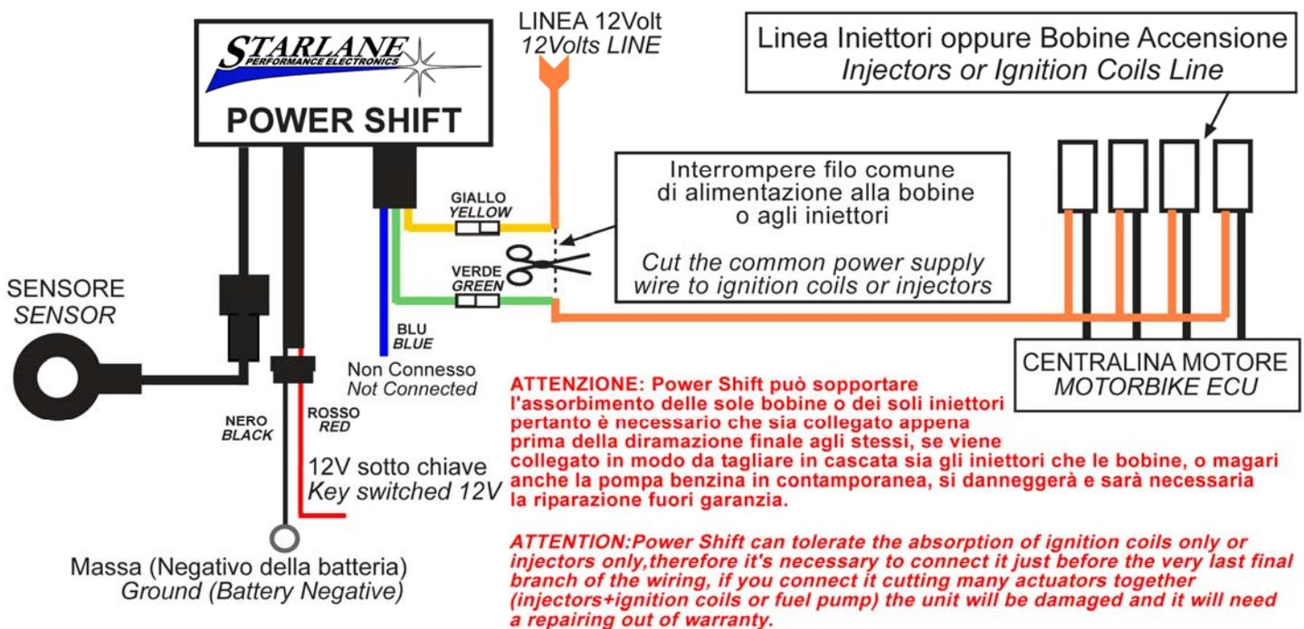
**COLORAZIONI PIÙ DIFFUSE PER IL TAGLIO DELLE BOBINE - MOST COMMON COLORS FOR IGNITION COIL CUT**
